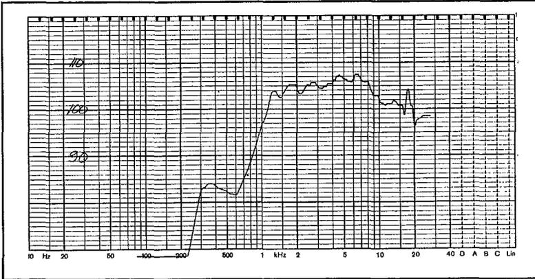
Figure 3.1 Sensitivity of the High Frequency Driver
