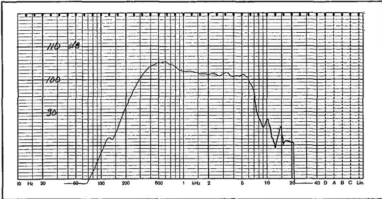
Figure 3.3 Sensitivity of the Midrange Driver in the Waveguide
