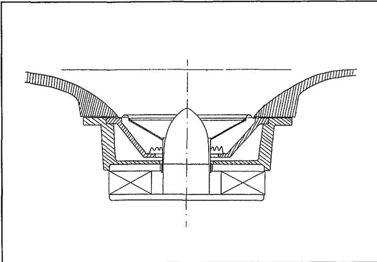
Figure 3.2 Midrange Driver Mounted on DCW Plate
