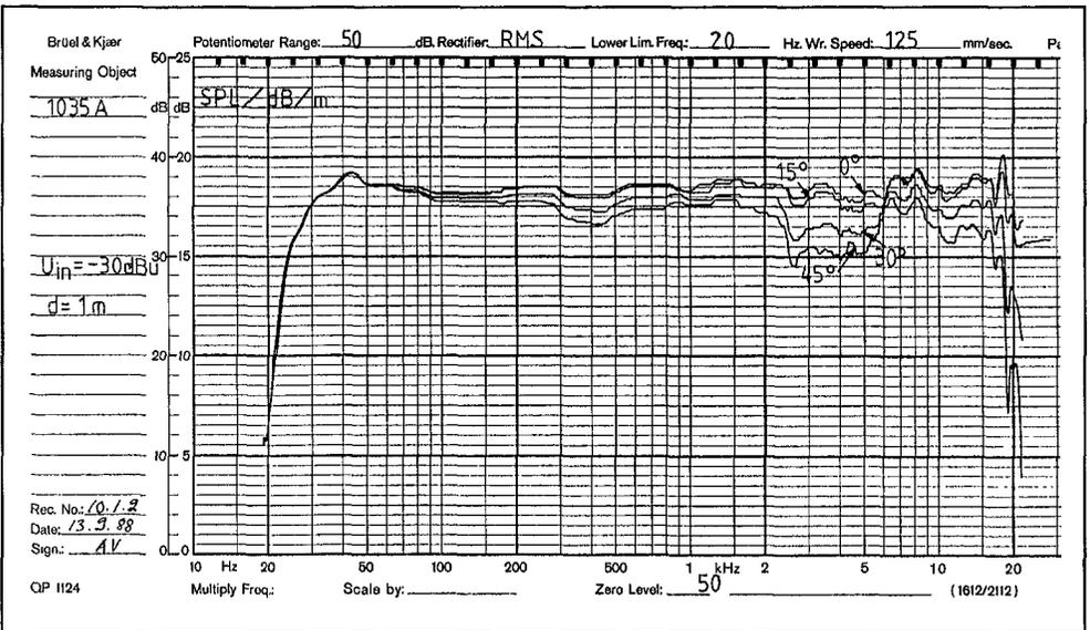
Figure 5.2 Frequency Response in Different Horizontal Angles
