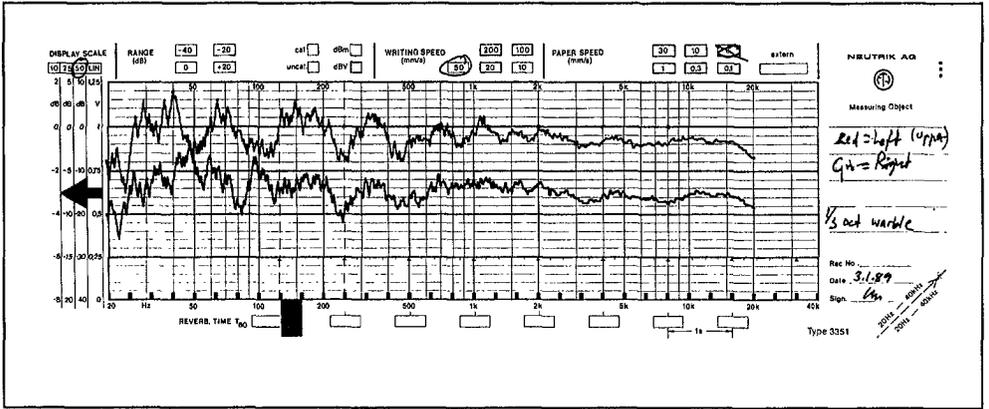
Figure 5.3 Frequency Response In Control Room
