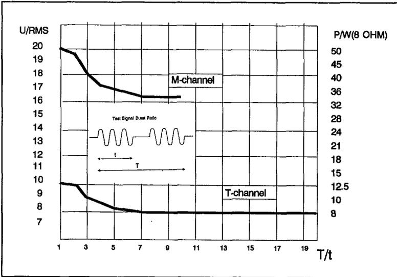
Figure 4.3 Maximum Continuous Power vs. Signal Burst Ratio
