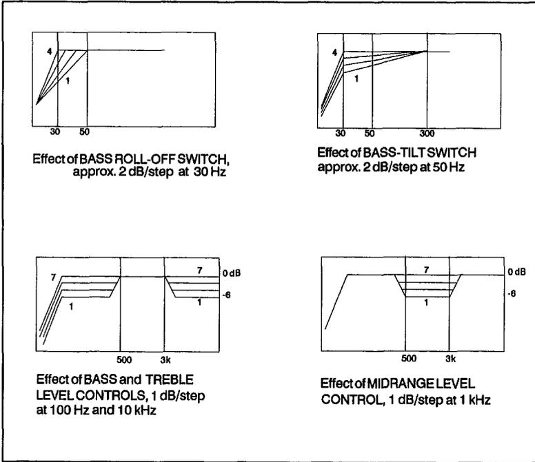
Figure 4.2 Effect of the Tone Control Switches
