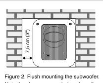
Figure 2. Flush mounting the subwoofer. Note the clearance needed on the reflex port side.
