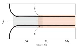
The Continued Directivity Mode uses the two woofers in the W371 simultaneously, to generate constant directivity which matches that of The Ones monitor being used with the W371. This creates a four-way monitoring system that has continued directivity on the horizontal plane right down to the lowest audible bass frequencies.
