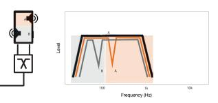
The Complementary Mode can circumvent any reduction in sound level at certain frequencies (known as 'acoustic notching') at the listening location, by placing the two independent woofers within the W371 at different physical locations in the room - and by then using the woofer that is best able to radiate audio to the listening location. In addition, GLM also equalises the W371 with The Ones for neutral audio, delivering uncoloured low frequency sound with great dynamics.
