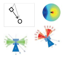
The Anti-reflection Mode uses the two woofers in the W371 simultaneously to generate regions of silence (known as 'nulls') in certain orientations. These nulls reduce the levels of reflected audio in the operating frequency range of the W371 caused by various surfaces in the listening room. This also reduces the acoustic coupling of low frequency energy into room reverberation, thus reducing any detrimental effects of the room's acoustics.
