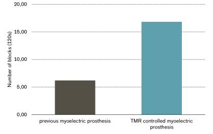
Performance of the pre-surgical myoelectric device and the TMR controlled myoelectric prosthesis was compared with a modified Box and Blocks test (patients were standing instead of sitting while the duration of the test was increased to 120s instead of 60s). With the new prosthesis patients showed marked improvement (on average 177%)
