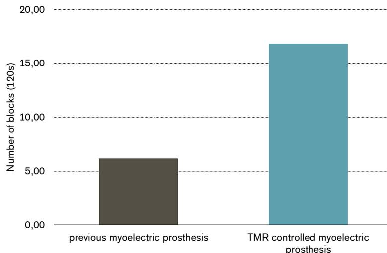
Performance with the pre-surgical myoelectric device and the TMR controlled myoelectric prosthesis was compared with a modified Box and Blocks test (patients were standing instead of sitting while duration of the test was 120s instead of 60s). With the new prosthesis patients showed marked improvement (on average 177%) (Miller et al., 2008)
