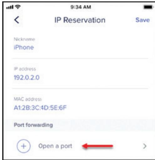
7. Fill in the Port name, External and Internal port numbers, select the desired protocol, then tap **Save**.
