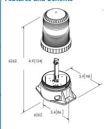
Reinforced nylon base is epoxy filled for environmental protection
