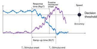
Figure 2.6: Illustration of the key variables for the heuristic model.
