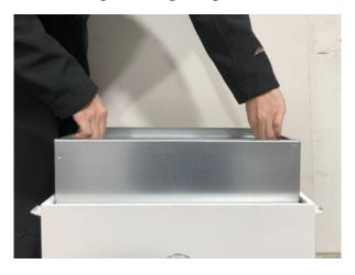
Lift the filter cartridge out
