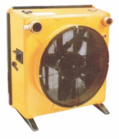
It is a high expansion foam generator. It consists of a fan driven directly by the shaft of the water turbine, which blows air to the nylon net. The net is wetted by foam water solution from the spray nozzle. The foam concentrate is drawn into the water stream by means of a built-in induction system.
