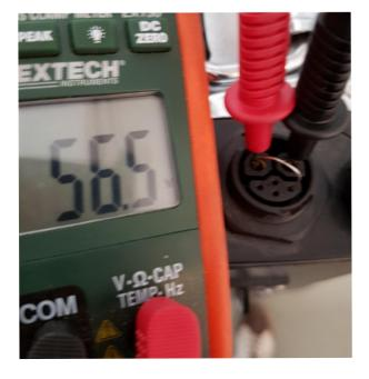
III. When you measure the voltage now again between pin 1 and 2, the multimeter should show a voltage around 50 V.
