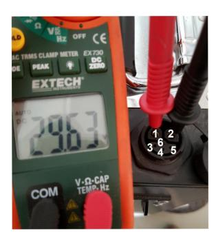
I. Normally, the voltage is measured only between pin 1 and 2.
