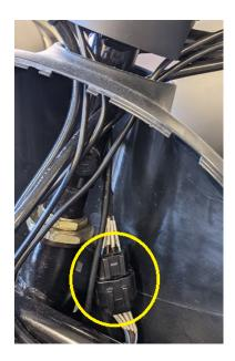
1.4.5. Checking the 16-pin connector and the USB cable (display must be remove from scooter for access)
