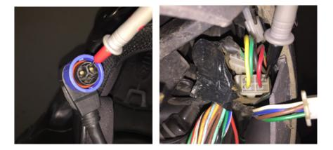
On the battery connector shown above, the pin on the multimeter carries the high-voltage signal that will later be connected to the enable line.
