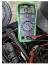
2.3. (2.2.6.3) Measurement of the charging current and voltage for charging the AUXB: Disconnect the + pole (red) of the AUX battery and measure the voltage against ground -> If no charging current or voltage are measured
