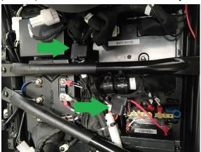
2.2. (2.2.6.2) Voltage measurement for the voltage between the DC converter and the 12 V system -> No voltage of 12V -13.5 V is measured at the output of the DC converter: Replace the DC converter SP-S-05-02-001
