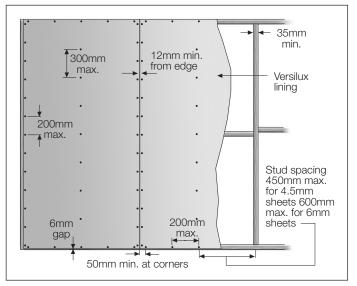
FIGURE 6 WALL FIXING
