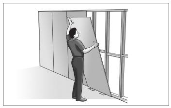
FIGURE 4 SHEET INSTALLATION
