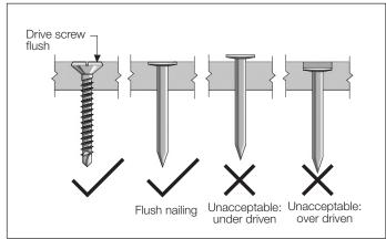
FIGURE 2 FASTENER DEPTH
