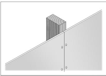
FIGURE 13 SHEET FIXING - BUTT JOINTING
