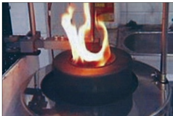
FIGURE 2: ALUCOBEST CATCHING FIRE IN NON-COMBUSTIBILITY TEST [3]
