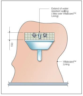
FIGURE 25 WATERPROOFING VESSELS ABUTTING WALLS
