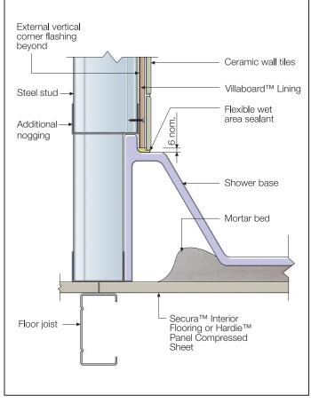
FIGURE 13B PREFORMED TRAY DETAIL FOR VILLABOARD<sup>™</sup> LINING TO BE TILED - STEEL FRAME
