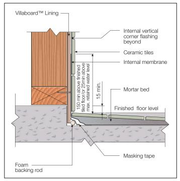
FIGURE 15A IN-SITU APPLIED INTERNAL MEMBRANE AT STEP-DOWN FIGURE 16 SHOWER OVER BATH - WITH SHOWER SCREEN - TIMBER FRAME OPTION
