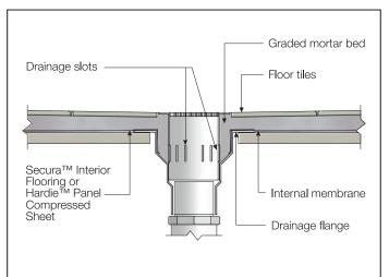
FIGURE 27 PRINCIPLE OF LEAK CONTROL WASTE
