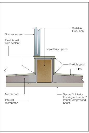
FIGURE 17 BRICK HOB - INTERNAL MEMBRANE
