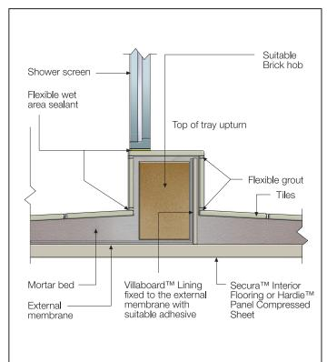
FIGURE 18 BRICK HOB - EXTERNAL MEMBRANE
