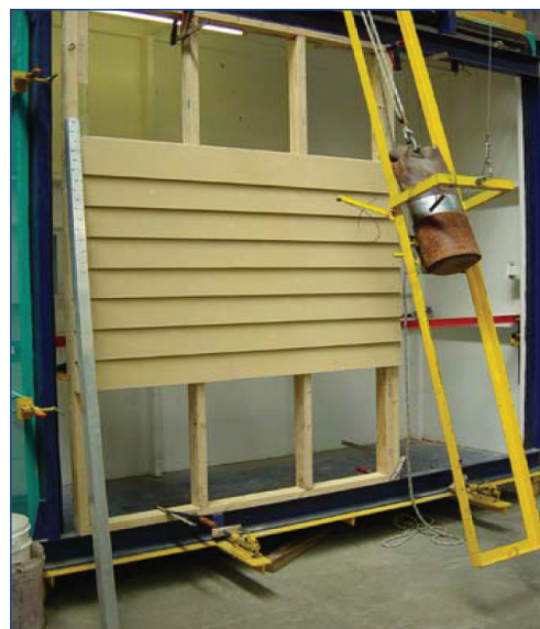
FIGURE 1 SOFT BODY SWINGING SANDBAG IMPACT TEST ON SCYON LINEA WEATHERBOARD
