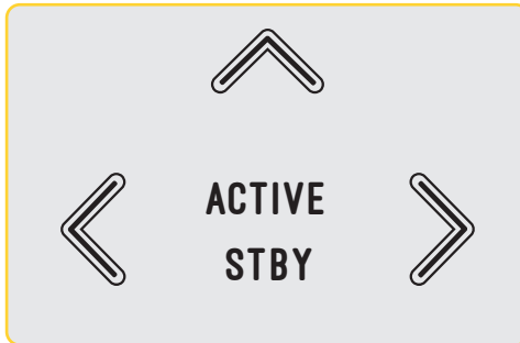
Press ACTIVE to initiate the Bluetooth connection between the laser unit and pedal
