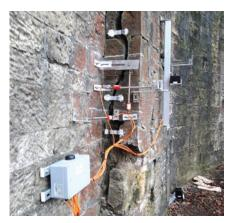
We installed six of our LVDT systems to provide 3D crack monitoring on either side of the pilaster. The system incorporates a specially designed mounting beam and anchor system, creating solid and permanent contact, measuring the X-, Y-, and Z-axes. The data feeds into DYWIDAG's cloud-based database, Infrastructure Intelligence, allowing bridge owners to better understand what is happening with the bridge.
