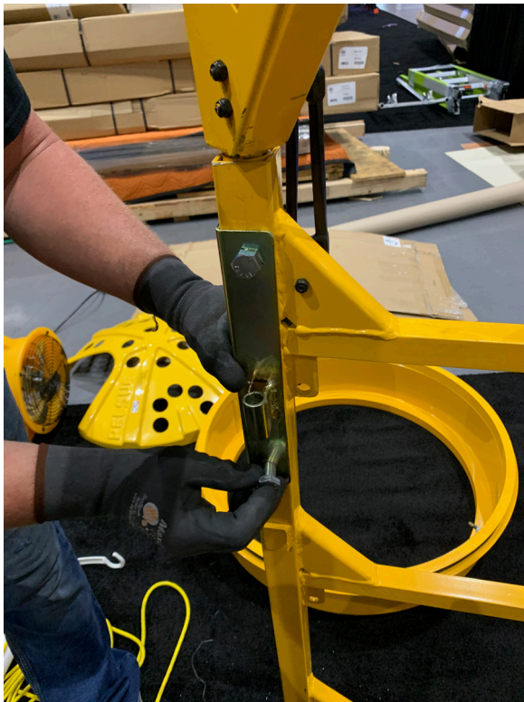
Figure 6: Install the spring latch receiver.
