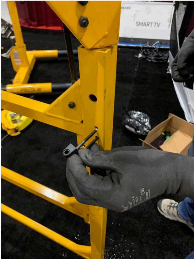
Figure 7: Install hinges using the included hardware.
