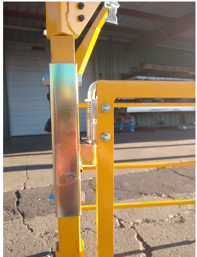
Figure 10b: Release the spring latch into the spring latch receiver.
