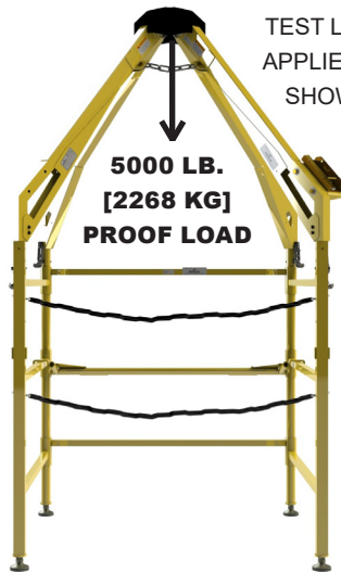
Figure 5.1b: LG5 Loading Diagram Configuration 1
