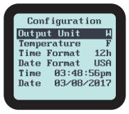
The DLM-4 Zone Controller unit has several configuration settings that can be customized by the user, those settings are stored in the Configuration page. Below is a description of the Configuration settings.
