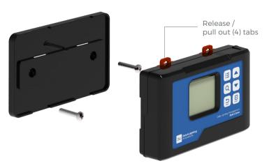
Determine where to locate the main controller. The controller comes with a simple to use DIN type bracket. Pull the 4 tabs outward to release the bracket from the unit, mount the bracket to a wall or surface, place the unit back on the bracket and press the 4 tabs back in to lock the unit in place.
