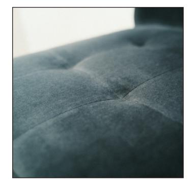
▲3 Due to the low elasticity of this fabric, wrinkles appear at seam lines.
