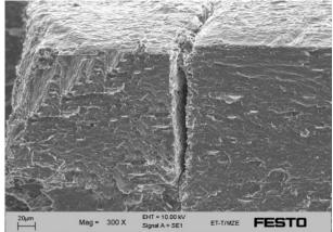
SEM micrograph of cracking in plastic
