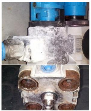
Incorrect choice of materials – typical damage profiles
