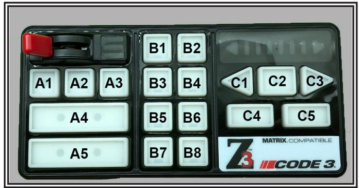
Figure 5 - Push Button Control Head Key
