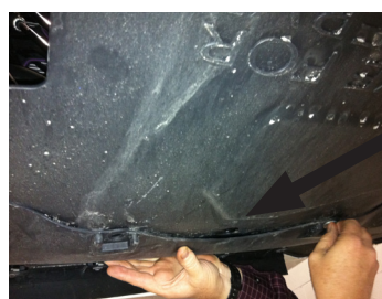
REMOVE 2 FRONT SCREWS FROM SKID PLATE
