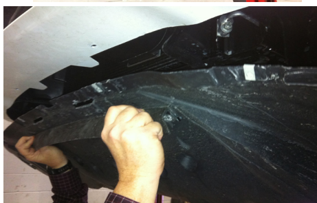
SLIDE SPLASH GUARD BACK AND REMOVE FROM VEHICLE
