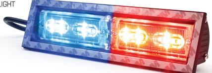
The CD3974 Series emergency warning light tightly mounts to interior windows using high bond tape. This low-profile, dual-color LED light is adjustable 7.5° up or down to accommodate a variety of window angles. Choose from four color combinations, each producing 67 flash patterns.
