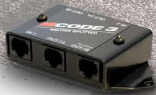
SPLITTER ENABLES 3+ MATRIX END NODES 10-32V / 1.0" H x 4.2" L x 2.1" D (2) CAT5 input ports, (4) CAT5 output ports
