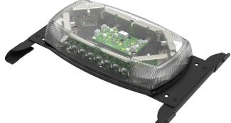
The universal CZ6015/CZ6016 Series drill-free rooftop mounting platform secures to the roof of any emergency vehicle using our high bond tape (HBT) technology, allowing warning devices like minibars, beacons, remote spotlights and full-sized lightbars to mount to the vehicle's roof without cutting into or damaging the cab. This no-drill rooftop platform installs in minutes and is made from industrial-grade aluminum.
