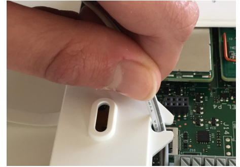
Insert the wire into the strain- relief
