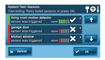
3 When all sensors have been tested, tap **OK**. Then continue with the Panel Test.
