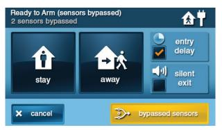
Sensor bypassing is also sometimes used when a sensor requires service. A sensor's magnet may be missing, or an external switch contact connected to a sensor may be faulty. This causes the sensor to report as **open** to the Control Panel.
