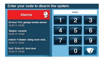
After the system is disarmed, the **Alarm Memory** screen appears. The **Alarm Memory** screen shows the sensor(s) that caused the alarm. If more than one sensor was triggered, the display shows the order in which the alarms occurred.
