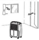
When moving or putting in storage, do not place the dehumidifier on it's side or upside down and avoid violent shaking.
