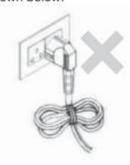
Make sure the plug is placed fully & firm into the socket.
