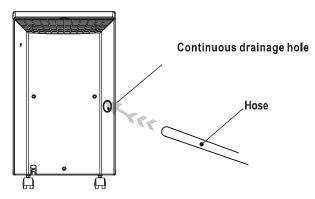
3) Put in the PVC hose through the hole, then connect the PVC hose to the internal drain pipe.
