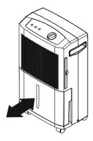
3) Turn the control knob to the suitable humidity position. If the indoor humidity is over the set humidity, then the machine will start removing moisture.
