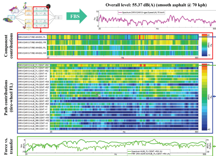
Figure 14. Typical results of a VPA calculation for road noise prediction.
