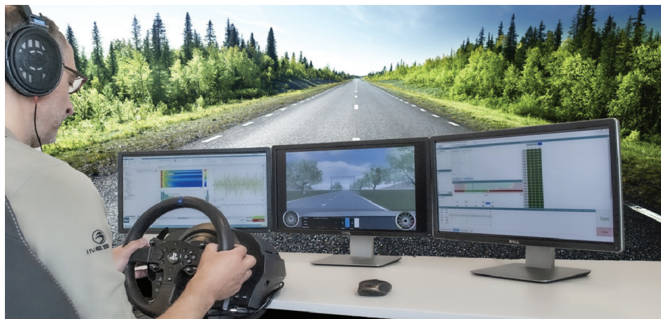
Figure 16. Evaluating sound perception in the early design stages with the vehicle sound simulator.
