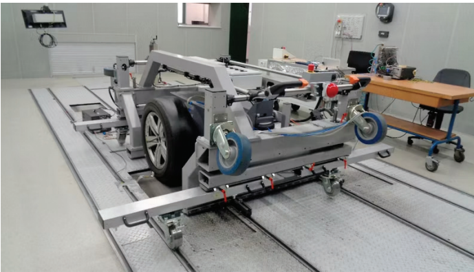
Figure 10. A tire force rig of an AZL to test front and rear suspensions and tire-rim combinations on the same excitations.
