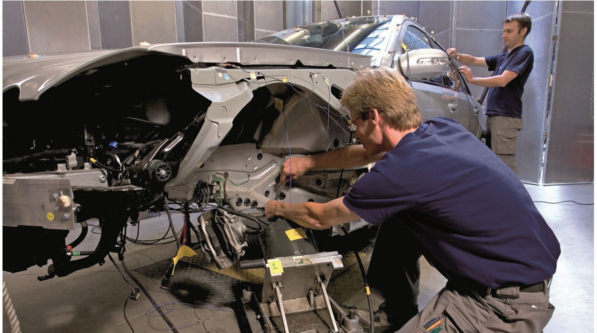
Figure 4. Engineers instrumenting the vehicle body for measuring FRFs at suspension mount locations.
