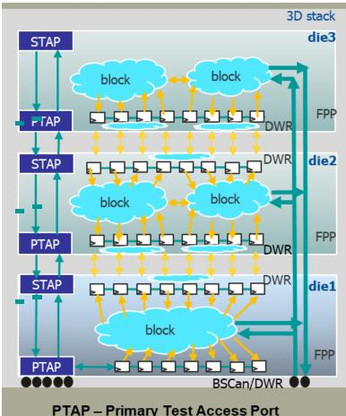
PTAP – Primary Test Access Port STAP – Secondary Test Access Port DWR – Die Wrapper Register FPP – Flexible Parallel Port
