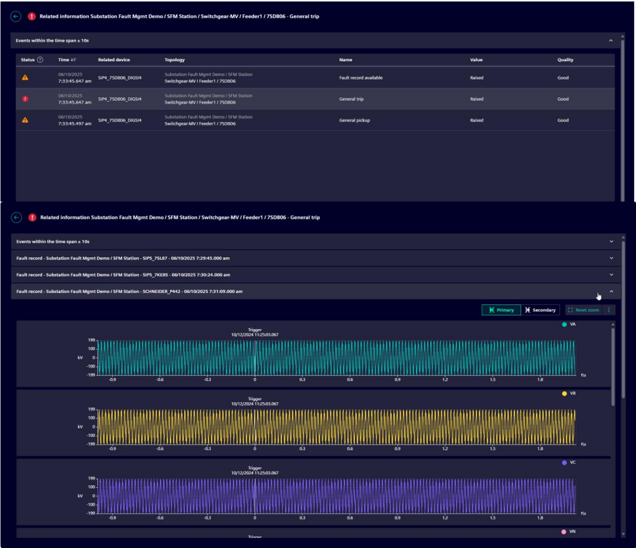
Electrification X – Network Fault Mgmt (Substation Fault Management): Aggregated information during fault
