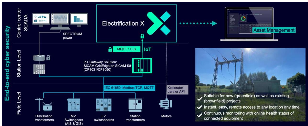
Data communication between the Connected Field Devices on premise and the Cloud Service requires internet connectivity (to be provided by the Customer).
