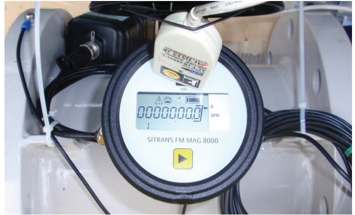
An infrared IrDA interface offers the ability to upload or download data via laptop.
