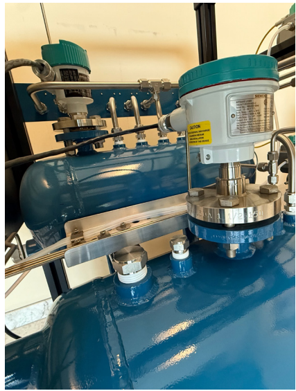
Left, the skid-mounted Xenon LRS Mini model. Right, a closeup of the Siemens SITRANS LC300 continuous capacitance transmitter in the foreground, with the SITRANS LVL200 point level switch in the background.
