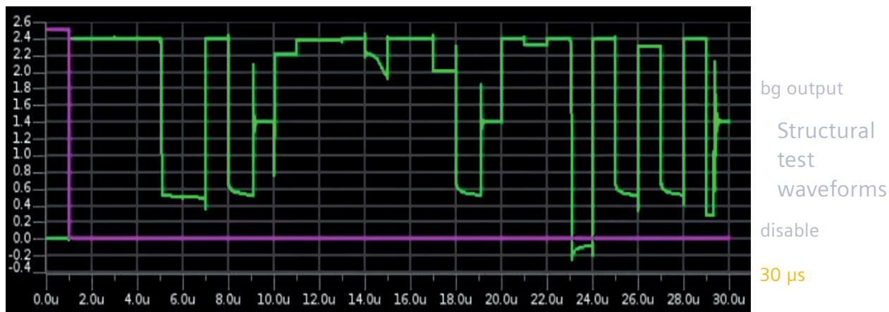
A single analog output during an example scan test.
