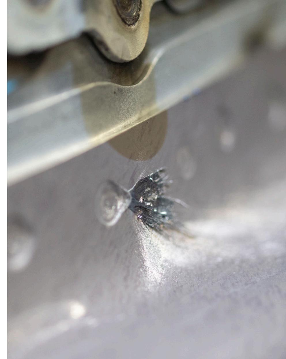
Audi's AI model uses blue light to highlight areas with weld splatters so workers can easily remove them
