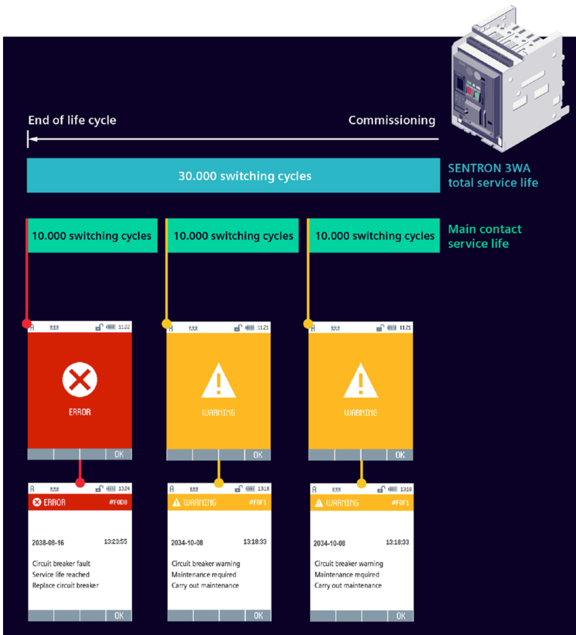
Figure 6: The system automatically sends warning and error messages to provide appropriate instructions.
