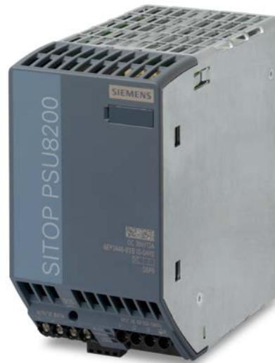
The SITOP PSU8200 is perfect for complex plants and machines. The wide-range input allows the connection to any network and tolerates large voltage fluctuations. Power Boost delivers up to 3 times the nominal current. In the event of an overload, you can choose between constant current with automatic restart and latching shutdown. And the high efficiency reduces energy consumption.
