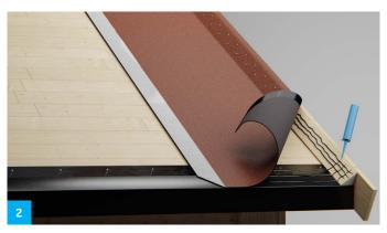
Apply three thick lines of Icopal Roof Glue to the triangular batten and roof fascia. Remove the tear-off strip from the underside. Spread TopSafe over the batten and the rake. Nail it to the batten. Cut the material against the eave fitting. Clean cut and check that the glue is leaking out at the eave fitting.
