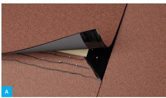
Measure an end overlap of 150 mm. If the drop is <3°, increase the end overlap to 200 mm. Apply glue generously to the end overlap and the cut area. The overlying part should be trod down and not nailed. The glue should leak out as a seal.
