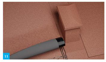
The Icopal Ventilation Hood with flange is fitted at the same time as the material. The ventilation pipe has a socket with  $\emptyset$  110, 125 and 160 mm connections. See fig. 10 for fitting of the ventilation hood. The glue should leak out as a seal.
