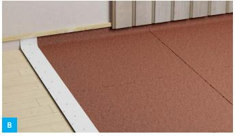
The material should be applied behind the cladding on dividing walls, min. 150 mm. N.B. Check that the material is stuck down sufficiently at the divide between floors and walls. If necessary, apply Icopal Roof Glue.
