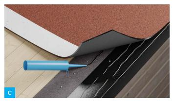
Finishing at the front edge of fittings. Use Icopal Roof Glue to seal fittings. Cut the material down against the fitting, see figures 2 and 7.
