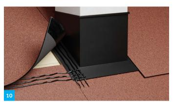
Cover up to the chimney and at least 50 mm past on each side. Put the fitting in place. To be on the safe side, apply 3 lines of glue under the material below the chimney. Lay TopSafe to the top edge of the pipe and down along the fitting, up to the chimney and approx. 50 mm below the flange. Apply Icopal Roof Glue to the fitting and the end overlaps. Tread down.
