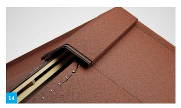
The gap in the ridge must be covered approx. 250 mm from the outer wall and 400 mm on each side in the case of a T-ridge. Apply a thick line of glue to each side under the ridge ventilation. Attach the profile with 6 screws. In locations exposed to harsh weather, a non-woven fabric must be laid over the gap to avoid precipitation collecting. The gap must be 50-70 mm.
