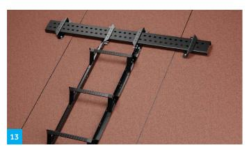
When fitting ladders, snow guards and similar to the roof, it is important to seal the screws under the mounting bracket with Icopal Roof Glue to prevent leakage.
