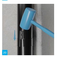
The pipe clamps are placed around the downpipe itself. Maximum distance between pipe clamps should be 3 metres. When using pipe clamps with a brick wall, use an 8 mm drill for the fastener holes. Carefully hammer the clamp lock into place.
