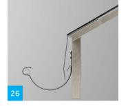
Steel table roof fittings are supplied in 2-metre lengths, the same colour as the steel guttering. Types BTS 2-23 and 3-17 are for stone/tile roof, type BPS 9-11 for asphalt roofing and roof shingles. Roof fittings should be mounted with an 8 cm overlap.
