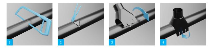
It is simplest to fit the downpipe spout on the ground. Mark where on the gutter the downpipe should be. Saw out a hole. Bend down the centre of the cut edge to create a drip edge. The front edge of the downpipe should be inserted into the lip of the gutter. Press the spout against the gutter and lock using the four lips around the back edge of the gutter.
