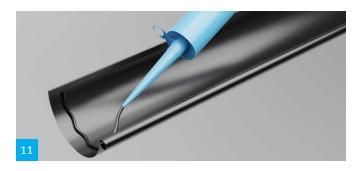
When joining gutters or angle pieces, bend the rear edge up approx. 6 cm on one gutter. Apply sealant.
