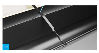
Gutter supports are used where there is a need to fit beside hooks, e.g. to follow the AeroDek profile or where adjustable gutter hooks are used. When using gutter supports, there is a risk that water will flow along the gutter support and over the gutter.
