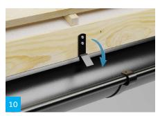
Joint piece: Move the gutters all the way together and make sure they are at the same level. The rear edge of the joint piece should be hooked into the rear edge of the gutter and pulled sharply downwards. Then the front edge of the joint is pressed in over and in contact with the folded edge.
