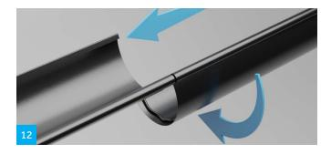
Then gently turn the gutter and push together. The folded edges at the back should be squeezed together with pliers. See figure 15.
