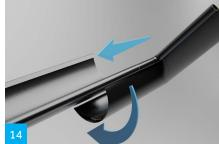
Apply sealant to the gutter angle and rotate so it comes into contact with the gutter. As an alternative, a joint piece can be used, but gutter hooks must then be fitted to the angle to hold it in place.
