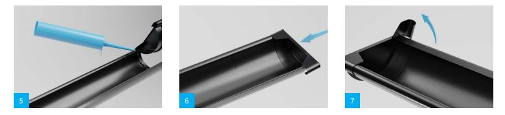
Fit the end cap into place before installing the guttering. The end cap will fit at both ends. Break off the folded edge towards the back edge of the gutter. Twist the gutter piece into the folded edge. Apply sealant to the inside of the gutter. Then bend in the back lip. The distance between the end cap and rake should be 10-15 mm.
