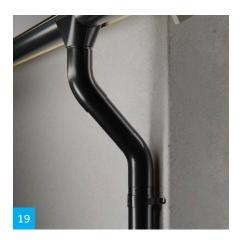
The middle piece should be lowered into the lower bend and then inserted onto the top of the upper bend. Fit the downpipe. Shrinking tubing is only used when the downpipe is joined.
