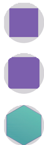
Figure 12: To cut the monocrystalline round wafer hexagonally provides more efficiency in material use and module lay-out
