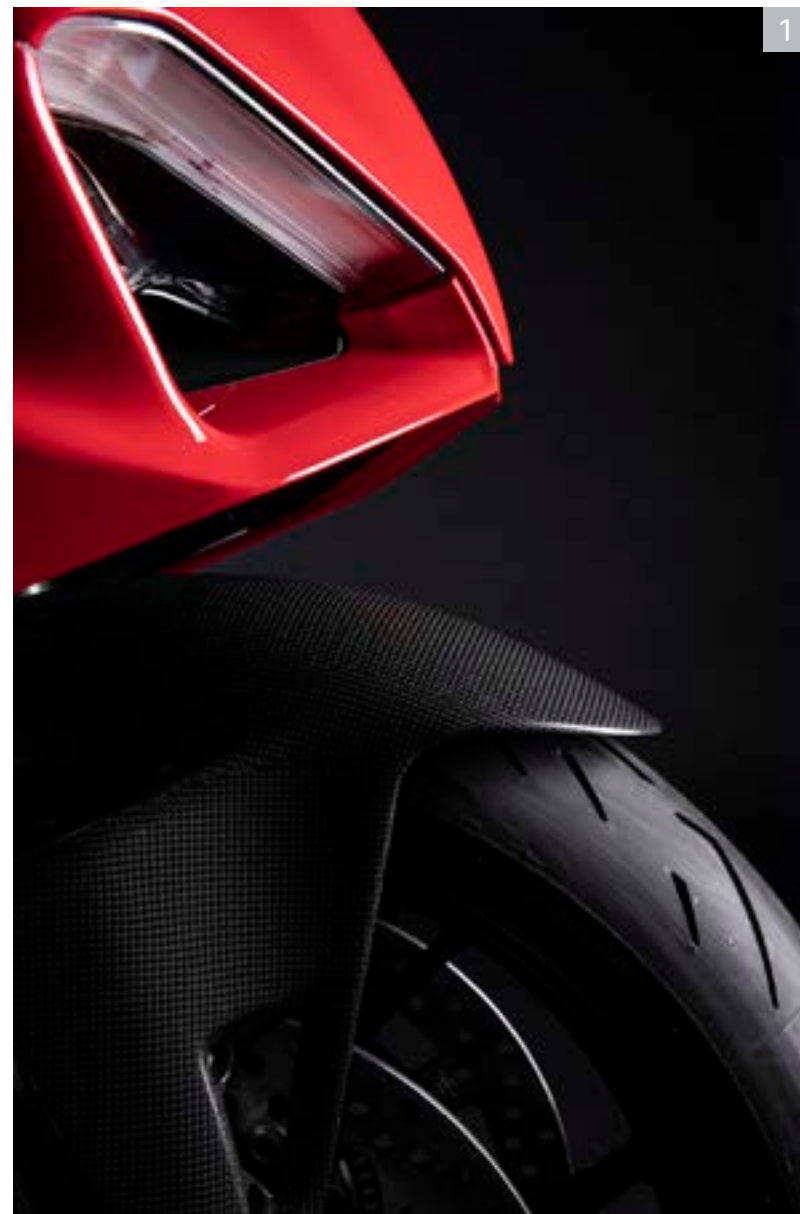
1 Carbon front mudguard.
