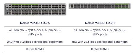
The QSFP-DD ports also support native 200G (QSFP56), 100G (QSFP28) and 40G (QSFP+). Each port can also support 4x10G, 4x25G, 4x50G, 4x100G, and 2x200G breakouts.
