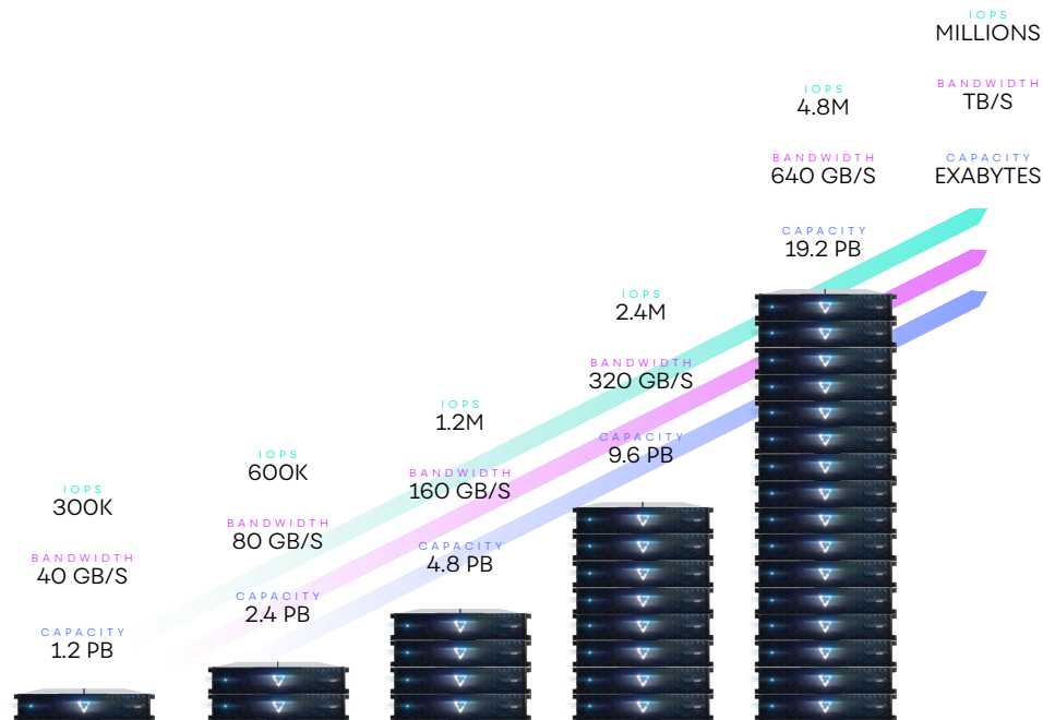
Figure 7 – VAST Data scales performance linearly with affordable 100% NVMe-flash systems
